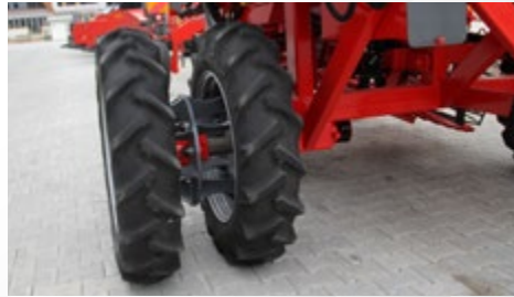
ÇİFT TEKER SİSTEMİ DOUBLE WHEEL SYSTEM
