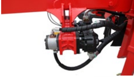
3'LÜ POMPA SİSTEMİ 3 PUMP SYSTEM
