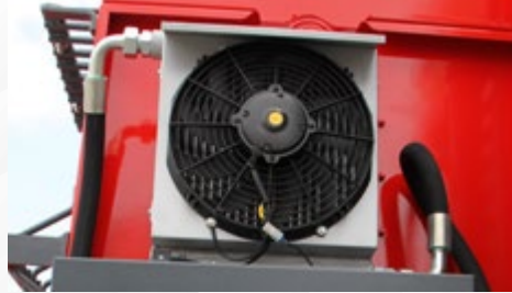
YAĞ SOĞUTMA SİSTEMİ OIL COOLING SYSTEM
