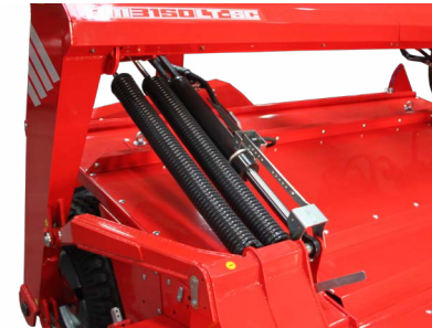
ENGEBELİ ARAZİDE AYARLANABİLİR TABLA ADJUSTABLE TABLE ON ROUGH TERRAIN
